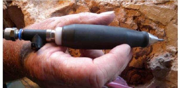
HW-70 Tips - Pointed and chisel shapes available in regular and extended lengths.
