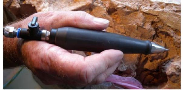
HW-65 Tips - 3mm diameter - Pointed and chisel shapes available in regular and extended lengths.
