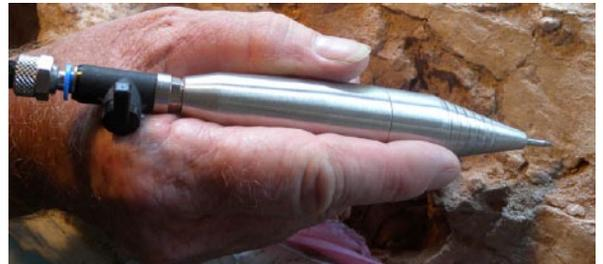
HW-90 Tool (the beast) This is the biggest and strongest for big jobs. It works great on hard matrix. Largest tool you can use in one hand allowing use in glove box. Comes with an inline regulator (see photo HW-323). Pressure should not exceed 4 bar (approximately 60 psi) otherwise the tool would destroy most tips. Max 4 bar.
