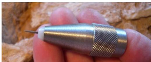
HW-10 Head with needle holder (micro adapter for the Aro airoscribe) plus 1 extra carbide tip and five steel tips. Runs at 2.5 - 6 bar.
